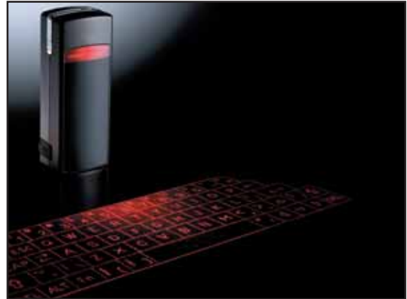
Fig. 9 Virtual keyboard using Bluetooth and laser-projection technologies (courtesy of i.Tech Dynamic Limited, Hong Kong; www.itechdynamic.com ).
